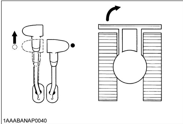
2. Pull the left drive lever backward; the excavator will turn in the direction of the arrow of the illustration below.
