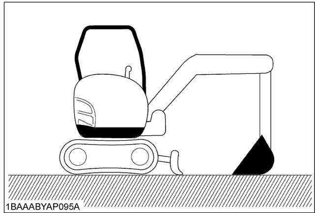
2. Remove the drain plug on the underside of the hydraulic tank and drain the oil.
